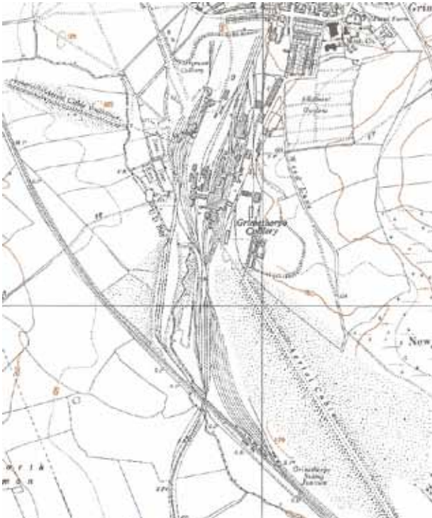
Ordnance Survey map from 1955 showing the growing footprint of the colliery including railway sidings and the aerial cables leading to spoil heaps From the RGS-IBG Map Library
